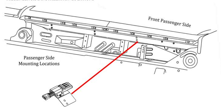
**Step 5**: Install the control module on passenger side using (2) M8X30mm Flange Bolts, to fasten the motor to the vehicle. Use the center rear mounting location. The hardware should be hand tightened only until snug. This will allow the motor assembly to move and align easier when installing the running board.
