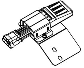
**Notice:** As shown in the picture, there is a four conductor plug, a six-conductor plug, a black two conductor plug, and a red two-conductor plug.
